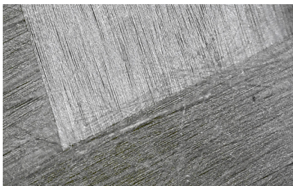
LAMINATE WITH E GLASS SURFACING VEIL
